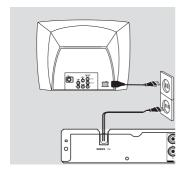
After everything is connected properly, plug in the AC power cord to the power outlet. Never make or change any connections with the
